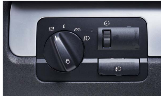
Light switch on LSZ (shown in "A" position)
